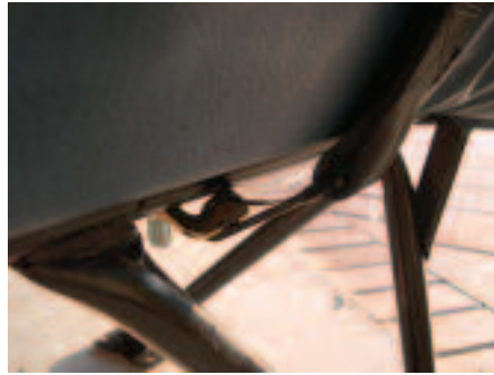
Tether anchors under bus seat using seat belt hardware and an E-Z-ON swivel bracket
